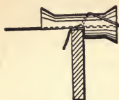
FIG. 7.—METHOD OF HOLDING GRADE-CORD.
